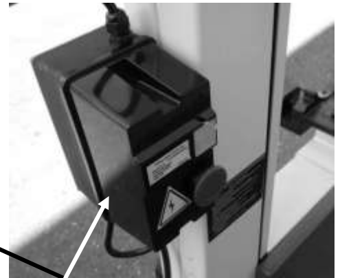
Switch in operation position
