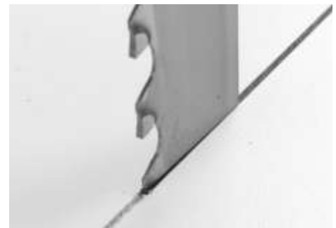
Blade not centered in saw cut
