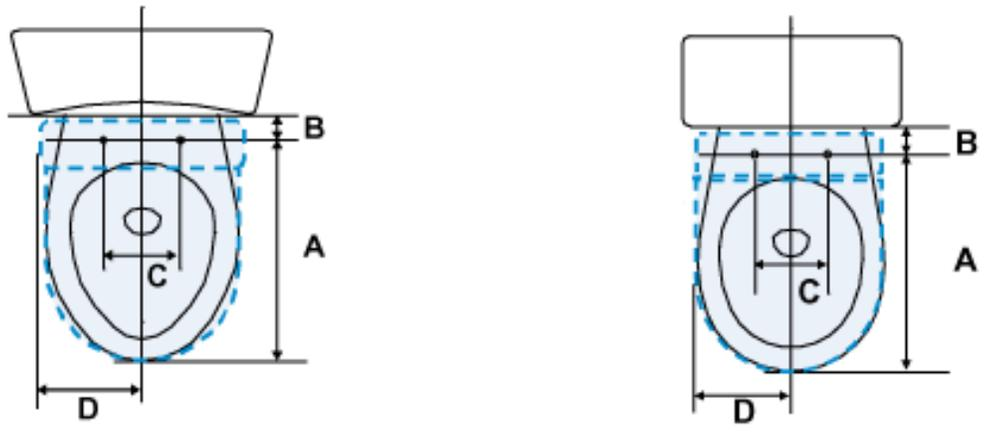
**Note:** Some styles of toilets may not allow the Washlet S300 to be installed due to certain contours near the tank and bowl area (see figures below). In the figure on the left side below, dimension D does not allow for enough open space to accommodate the minimum width of 9 inches.
