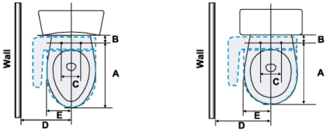
**Note:** Some styles of toilets may not allow the Washlet C100 to be installed due to certain contours near the tank and bowl area (see figures below). In the figure on the left side below, dimension D does not allow for enough open space to accommodate the minimum width of 12-1/2 inches.
