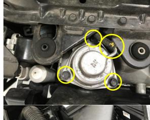
8. Disconnect Plumb back hose and remove lower portion of the factory BOV
