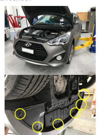
2. Unscrew all fasteners from the bottom of the front bumper.
