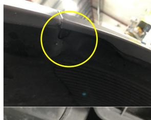
4. Pull the splash guard away from the bumper to gain access to the back of the fog lights, carefully unplug the connector.
