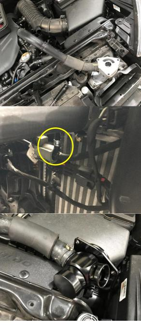
11. Install your new Turbosmart BOV in the factory location. NOTE: Ensure that the BOV flange has Oring in place prior to installation. Use the supplied M6 bolts to secure BOV. Torque to 6 Nm (4.23 ft.lbs). Install hose onto BOV fitting
