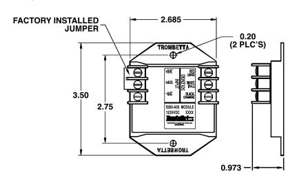
NOTE: When using a S500-A50 module all of the solenoid connections must connect to the module as shown.
