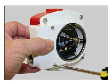
Remove the two (2) small screws from the front of the instrument.
