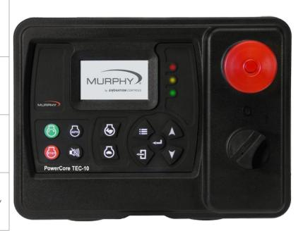
Murphy's PowerCore® TEC-10 panel provides full control of your engine including auto start/stop, auto throttling and display of engine parameters along with critical faults from the engine/application. The TEC-10 supports SAE J1939 CAN protocols for electronically governed engines as well as analog sensors on mechanical engines for fault and safety warnings/shutdowns.
