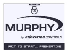
**NOTE**: The above screen will not be displayed for mechanical engines.
