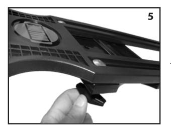
Loosely thread the two T-knobs onto the Bolts. Slide the Frame forward towards the Mounting Plate until travel is stopped. Tighten both of the T-knobs. See image 5.
