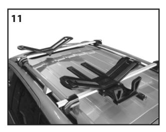
. Confirm the carriers are in alignment. Confirm that the mounting bolts are tight and both carriers are securely fixed to the cross bars. See image 11.
