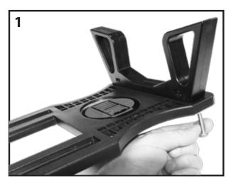
. Insert the two 1" bolts into the two holes located on the bottom side of the Extension Frame. Tighten with a Phillips screwdriver. See image 2.
