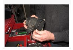
19. Install the MAF Adapter (B) into the S&B air box (A). Make sure it is aligned properly.
