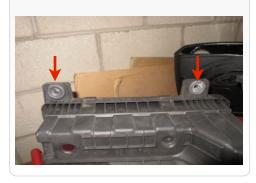
16. Push both grommets into part (K) Mounting Brackets. Put brackets to the side which will be used later in the install. Note: placement of the grommet in the bracket is with the large end facing downward.
