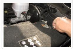
Remove the factory engine cover by pulling up and out.
