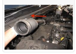
$8.\,\,$  Remove the lid by first removing the latches on the side of the factory air box.
