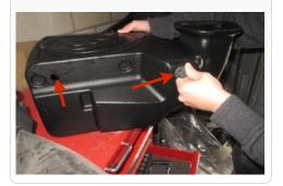
**15.** Remove the grommets from the factory air box side tabs.
