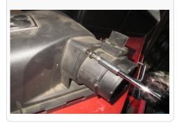
**18.** Also remove the rubber O-ring from the factory MAF.
