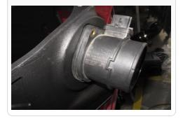
22. Use the provided hardware (D,E,F) to mount the factory MAF onto the S&B air box.
