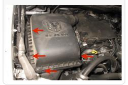
9. Remove the air box lid by lifting up and out
