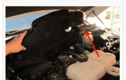
3. Disconnect the MAF sensor harness by pulling out the red latch and pushing down on the release button and pulling out.
