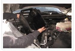
29. Use the provided hardware (L&M) to attach the S&B air box to the brackets.
