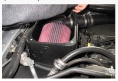
35. Install the Lid (N) onto the S&B air box using the provided hardware (P&Q) and the install is complete. Please make sure all hose clamps and hardware are tightened.
