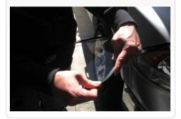
34. Install the S&B Filter with Adapter and tighten down Hose Clamp (H) on the MAF Adapter. Note: Make sure the Filter Adapter is fully inserted into the MAF Adapter, also make sure the top of the filter is just under the top of the air box.
