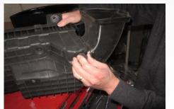
14. Install both grommets on the bottom of the S&B air box.
