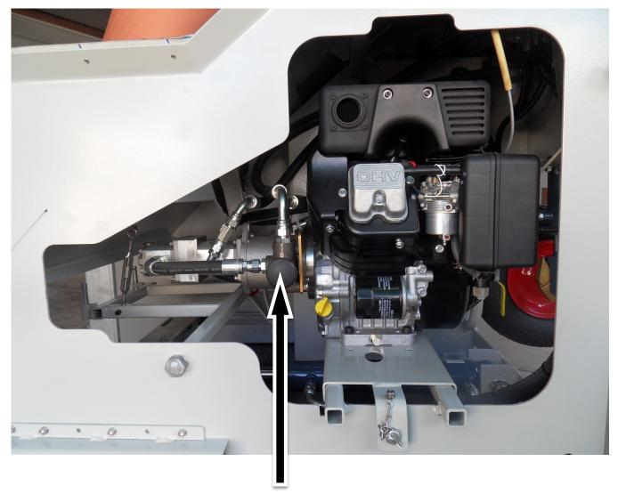
Use this selector to change pump selection Pull out for single pump operation or push in for dual pump operation.
