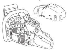
Remove the air filter after taking off the air filter cover.
