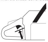
Press the throttle lock and make sure it returns to its original position when you release it.
