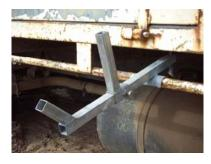
If rolling the pipe is not convenient cuts may be done <sup>1</sup>/<sub>4</sub> at a time by moving the tool on the stationary pipe and then rotating it between cuts.
