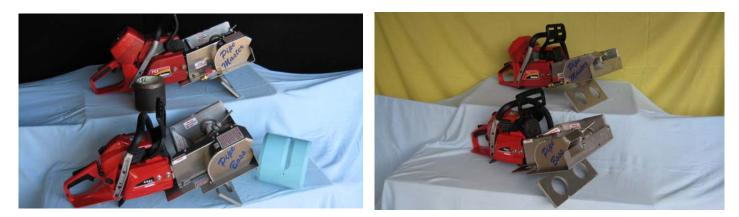
Whenever possible use the truck brackets or a similar support system for ease of operation. Heavy or large pipes will have to be worked on the ground using pipe rollers.
