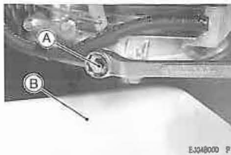
A. Oil Drain Plug (On side of engine) B. Container
