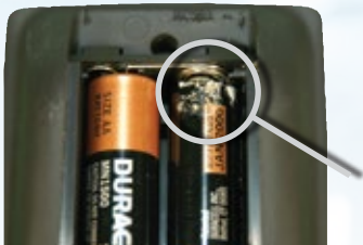
Corrosion you CAN see
