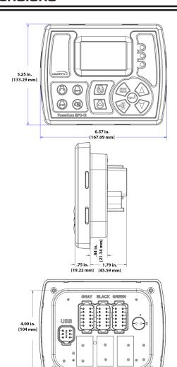
4X 6-32 UNC - 2B X 3/16 MAX DEPTH STAINLESS STEEL INIGEDT
