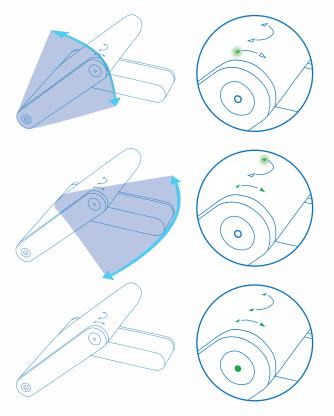
Tilt your iSavi™ up or down in the direction of the flashing green light until both 'up' and 'down' LEDs are solid green.
