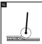
Roll flooring with a 100 lb. (45 kg) roller within 1 hour after installation to complete the bonding process.
