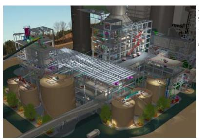
When Utility Engineering, Denver, was designing this gas desulfurization system with a wastewater treatment system at coal-fired power generating plant in Roxborough, N.C., designs were changed in the model before procurement errors and installation conflicts were encountered, which helped minimize interferences and eliminate redesign and construction rework.
