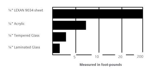
¶) Drop Dart Test with a 5-lb steel dart and a 1" diameter tip.
