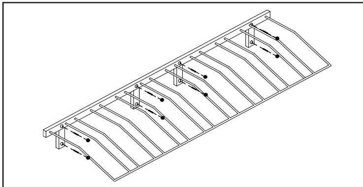
2.1 Align the WS-PR below the WS Series Wall Strips and make note of the Wall Strips that correspond to the Mounting Braces of the WS-PR.
