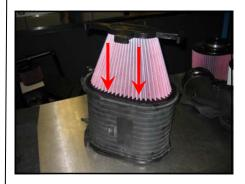
11. Be sure that the base of the filter is pushed down to the plastic "webbing" and seal is complete.
