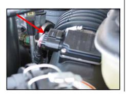
5. Loosen the hose clamps on the air induction tube
