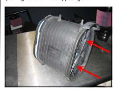
10. Install the S&B High Performance Filter into the open end of housing as shown. The fit is very tight. Use a small amount of soapy water to aid in installation if necessary.
