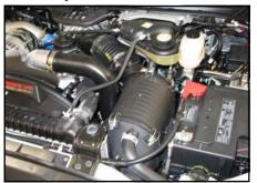
2. Disconnect the radiator overflow. Make sure the system is cold. The tube is under pressure
