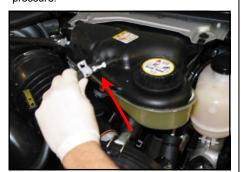
3. Disconnect the electrical connection for the air filter gauge.
