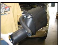
7. Isolate the filter core from the OEM intake tube and OEM snorkel by unclasping the clasps.
