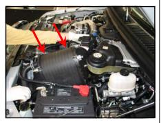
15. Tighten the hose clamp at the turbo manifold. Reconnect the electrical connections for the MAF sensor and the Air Restriction gauge.
