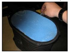
9. Remove the filter from the housing by pushing it out from the opposing side.
