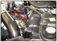
6. a) Remove air induction tube and lift out the OEM air box assembly from the vehicle.
