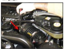
16. Reinstall the radiator overflow line.
