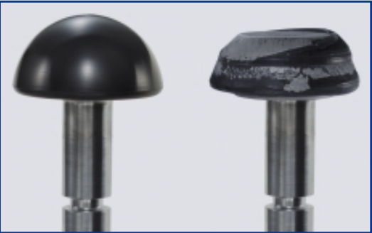
Metal detectable elastomers, if worn or broken off, can now be easily identified with in-line metal detection.
