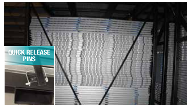
SAFETY SWING ARMS KEEP PANELS IN PLACE
