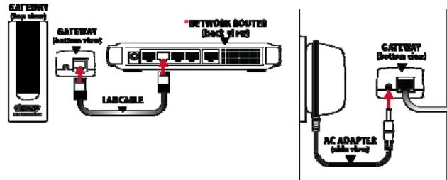
\*Your network router may look different than the diagram. Locate an available port on your router and plug in the included LAN cable. If you do not have a router, please visit [www.weatherdirect.com/router](http://www.weatherdirect.com/router).
