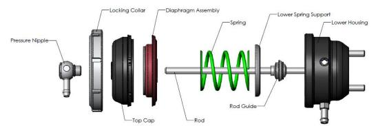
**IMPORTANT:** A press or clamping device must be used when removing or installing the collar as clamping the cap down removes the load off the collar from the diaphragm and allows the collar to be removed.
