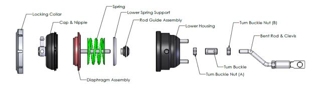
**IMPORTANT:** A press or clamping device must be used when removing or installing the collar as clamping the cap down removes the load off the collar from the diaphragm and allows the collar to be removed.
