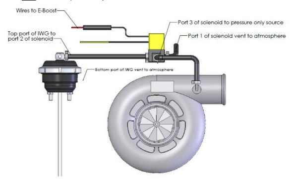
Two port connection (For controlling boost on a turbo system with high back pressure)
