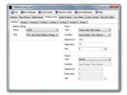
Analog Inputs - Analog 0, Battery Voltage
