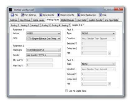
Analog Inputs - Merged tabs 6 & 7 when Thermocouple is selected
