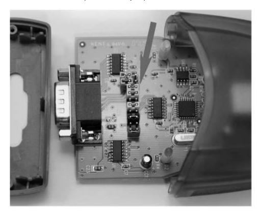
This RS485 Converter printed circuit board contains only jumpers.
