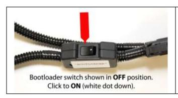
Verify Bootloader switch is OFF, and then turn the main power **ON** (click the power switch to the **ON** position).
