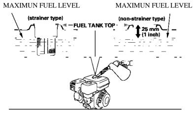
Refuel in a well-ventilated area before starting the engine. If the engine has been running, allow it to cool. Refuel carefully to avoid spilling fuel. Do not fill the fuel tank completely. Fill tank to approximately 25 mm (1 inch) below the top of the fuel tank to allow for fuel expansion. It may be necessary to lower the fuel level depending on operating conditions. After refueling, tighten the fuel tank cap securely.
