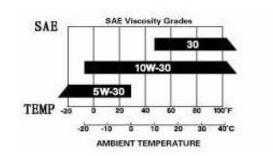
or equivalent. Always check the API service label on the oil container to be sure it includes the letters SJ, SL, or equivalent.
