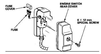
Frequent fuse failure usually indicates a short circuit or an overload in the electrical system. If the fuse burns out frequently, take the engine to a servicing dealer for repair.
