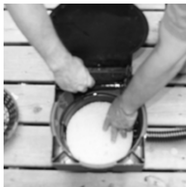
D) Insert filter pad.
