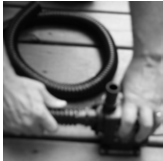
B) Push tubing onto hose barb.
