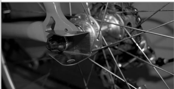
6. Insert the straight end of this 3-piece bar into the short adapter bar. Secure in place with a baled lynch pin.
