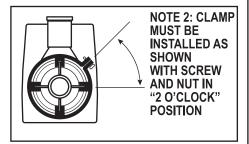
NOTE 3: The two protruding tabs located on the inside surface of the Ring Clamp must be inserted into the two slots on the outside diameter of the Motor Housing before
