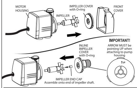
**NOTE 1:** If Impeller end cap remains attached to Impeller cover when removing the Impeller Cover, it must be removed and reassembled onto the impeller shaft. Insert impeller into the opening in the motor. Be careful, the powerful magnet may pull the impeller very quickly and possibly injure your finger tips.
