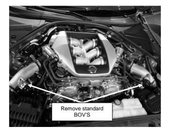
2) Install the Dual Port BOV's using the standard bolts. Remember to put in the provided gaskets between the flange and the BOV. Replace the plumb back hose and secure with the standard clamp.
