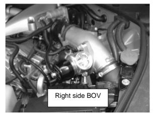
3) Replace the standard vacuum lines with the hose provided in each kit. Use the spring clamps to secure the lines.
