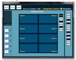
The Symetrix Room Combine 788's External Controller Wizard supports programming of Symetrix ARC Wall Panels for user control. While ARCs are simple and easy to use, you may prefer touch panel control. Symetrix now has interface templates available for SymVue.
