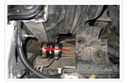
**11.** Place one the supplied T-bolt camps (I) over the Straight Coupler (H) and slide it on the upper end (Large diameter) of the Boost Tube (J).
