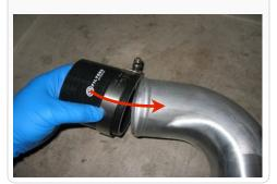
12. Snake the Boost tube assembly into position and into the Hump coupler (K).
