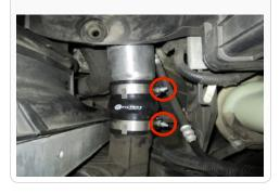
$14. \ \mbox{Place}$  the other supplied T-bolt clamp (I) over the end of the Straight coupler (H).
