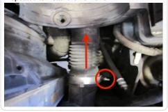
6. Remove the 4 bolts that secure the OE elbow to the intake manifold and remove the elbow from the vehicle. Be careful not to let debris fall into the intake manifold.
