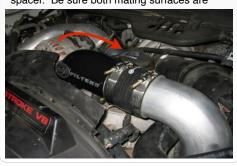
17. Insert the M6x30mm Bolts (F) and M6x93mm Bolts (E) in the proper locations and torque to 100 ln.lbs.
