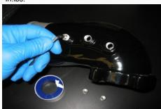
8. Place 6mm Washer (D) over each of the M6x30mm Bolts (F) and one over the M6x93mm Bolt (E), next apply a small amount of the supplied thread locker to each of the bolts.
