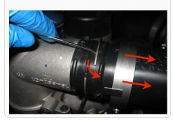
5. Loosen the hose clamp at the intercooler lower flange and remove the OE boost tube from the vehicle along with clamps. Remember how this is removed because it will have to be repeated to install the new one
