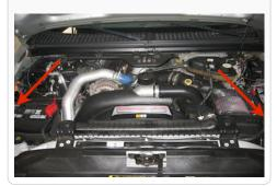
2. Optional step, to allow better access to the elbow. Use a small flat head screwdriver and pry the clips open and pull up working your way across to remove the upper fan
