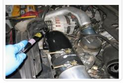
18. Position the upper T-bolt clamps as to not hit the hood when closed and torque them both to 90ln.lbs.
