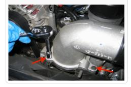
7. Apply sealant (Teflon tape) to each 1/8"NPT plugs (G) and insert the plugs into the ports you will not use on the elbow. Use 3/16" Hex drive and torque the plugs to 40 In.lbs
