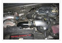
21. Reconnect both batteries. Inspect your installation, make sure the elbow and boost tube is properly positioned and all fasteners are secure. The installation is now complete.
