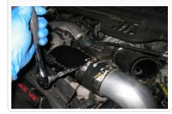
**19.** Reinstall the Intake or OE air cleaner and filter removed in Step 3.
