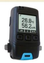
The EL-GFX-2+ standalone USB data logger measures and stores up to 252,928 temperature and humidity readings over a -30 to +80°C (-22 to 176°F) and 0 to 100%RH range at a resolution of 0.1°C (0.1°F) and 0.1%RH.
