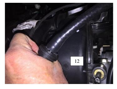
13. Once installed, the boost reference adapter and hose should look as shown.
