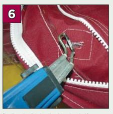
Sealing the fabric slit with a hot knife.
