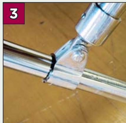
Mark the position of hardware before disassembly.
