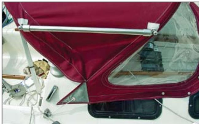
*In less than an hour a grab rail can be added to any 1" (25mm) diameter frame that can be disassembled.*
