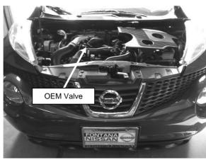
2) Remove the OEM valve by carefully removing recirculation hose, vacuum hose and mounting screws.
