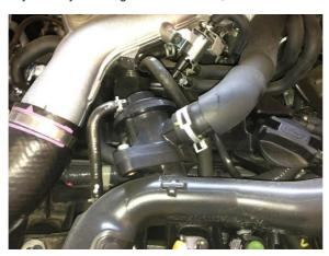
3) Install the Turbosmart Kompact valve on the flange, remember to install the provided gasket between the flange. Reinstall the OEM recirculation pipe and secure it with the OEM hose clamp.
