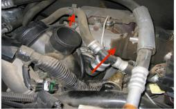
8. Install the Turbo Mouthpiece (A) onto the turbo inlet using the OE V-band clamp. Be sure both flanges mate in the V-band clamp evenly. Leave the connection slightly loose for now.
