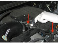
4. Using a 10mm socket, remove the screw mounting the CCV tube on the passenger side.
