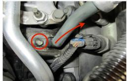
7. Loosen the V-band securing the OE inlet tube to the turbo. Then remove the OE inlet tube from the truck.
