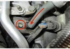
12. Use the supplied wire tie to position the small wiring harness away from the turbo and mouth piece. Clip the CCV hose back into place.
