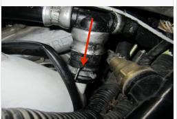
**11.** With the original O-ring in place, re-install the CCV line that was removed in Step #4 using the OE screw. Tighten using a 10mm socket.
