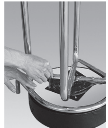
Step 4: Turn the bar stool over and secure the seat to the swivel with medium bolts as shown in the picture.
