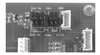
10. Reconnect all the plugs to the I/O board as shown below. The new I/O board supports only one hard wired remote. If your machine uses two hard wired remotes, one will have to be left unused.
