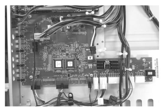
11. Install the new preamplifier and secure the mounting brackets using (4) Phillips screws left over from step 5.
