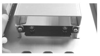
16. Install the SATA/PATA Converter, Item 4, and secure the board to the bracket with (2) 6-32 x 1/4" screws, Item 6.
