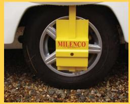
Slide the Milenco front cover with top strap over the wheel in a horizontal position, avoiding the wheel arch of the vehicle.
