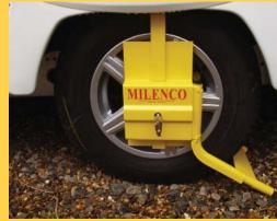
**Insert the right leg through** the right side of the front cover, ensuring the rear leg goes behind the tyre.
