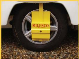
Rotate so that the top strap is over the centre of the wheel.
