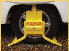
Insert the key and release the Insert left leg through the left side of the front cover. (Note: Lower edge of left hand locking plate must insert over right hand locking plate.)
