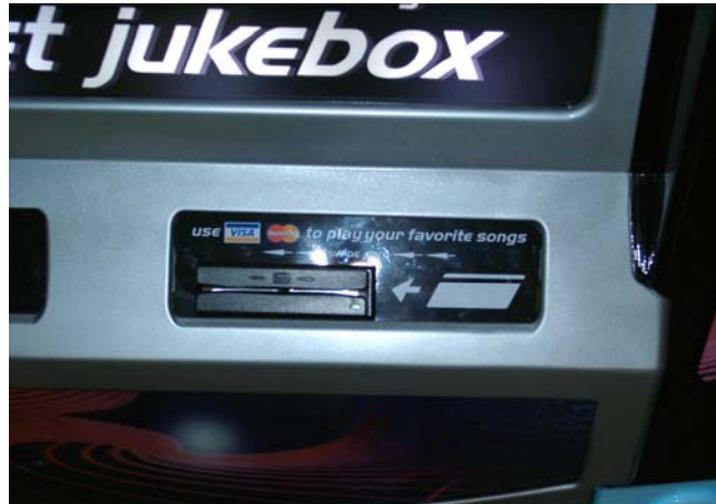
Figure 1.8-Credit Card Reader Installed
