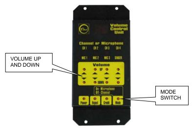
Figure 4 – Presetting the Microphone Volume
