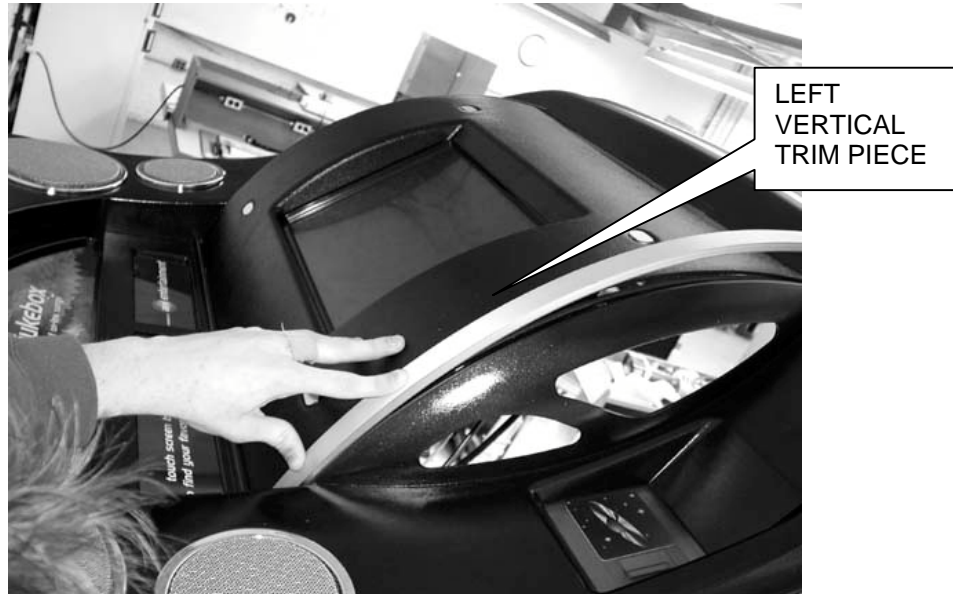
Figure 17 - Inserting Left Vertical Trim
