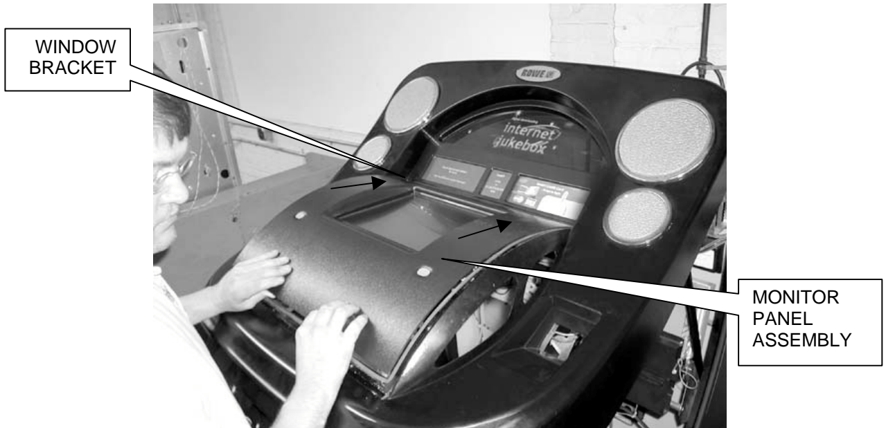
Figure 16 -Installing the Monitor Panel Assembly
