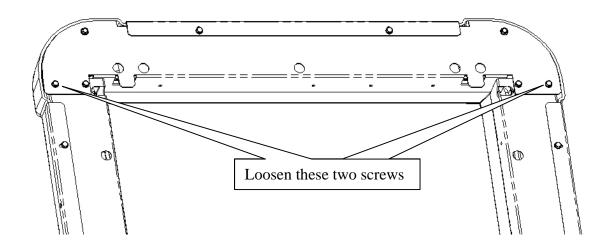
3. Place the Video Marquee Assembly (item 1) in position under the two loosened screws on the back of the lighting assembly then retighten the two Phillips screws. Drive (2) self drilling screws (item 5) through the holes on the back of the Video Marquee Assembly and into the top frame of the lighting assembly. Do not strip the screw holes as you drill.
