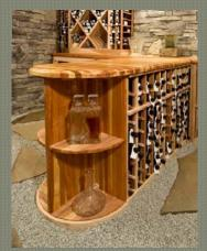
7) Quarter Round Shelves: Each shelf is dadoed (notched) into the sides and screwed into place from the back. The shelf is custom designed for equal centerlines on your shelves based on the overall height. You can select either solid, edge-glued material, or veneer plywood options for this item. The molding will be radiused to match the shelf or you can choose a square cut molding option for additional savings.
