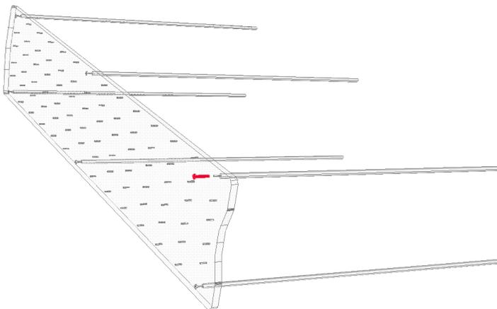
3. **Attach E1's to Remaining Holes in Panel** - Carefully lift the panel to stand on the unsecured ends of the E1's, like a table. Align the top of an E1 with a hole and pivot the rod into place and secure with an E1-SCREW. Repeat this process for the remaining holes.
