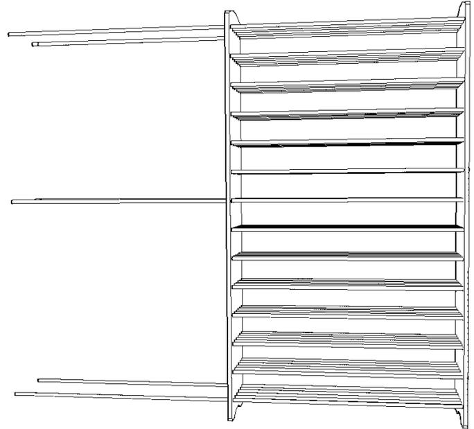
**6. Secure to Wall** – It is highly recommended that all units be secured to a wall for optimal stability. This may be accomplished by either directly fastening a panel to the wall by pre-drilling a hole through the panel and screwing or bolting into the wall or by using an "L" bracket. Please contact your VintageView dealer for information regarding brackets of custom shapes or sizes.
