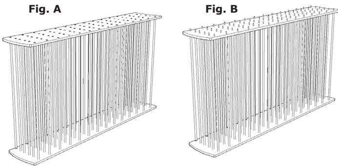
**5. Attach the E1's to Exposed Studs** (for Extensions only) – With all of the studs installed, begin securing the panel in place by installing E1's along the top, middle and bottom rows. Once the second panel is firmly locked in place, the unit may be stood upright for ease of access while installing the remaining E1's.
