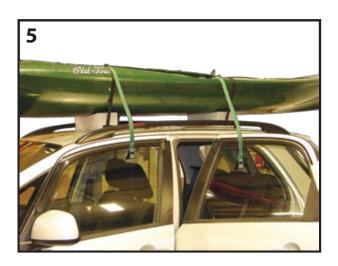
. With the doors open, pull both ends of the straps together and buckle from the inside of the vehicle. Confirm the straps are tight and secure. See image 6.
