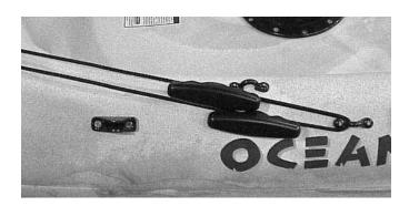
This is the trickiest part of the rudder installation. You may need to make tension adjustments so the rudder is neither too tight nor too loose for proper deployment and retraction. Keep the rudder assembly straight as you perform this installation—you may want help.
