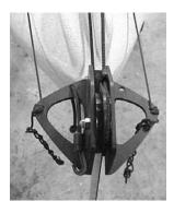
Keeping even tension on the steering line, (you may want help with this) secure it to the rudder housing. Make sure the housing is straight as you tie the steering line. Trim excess line with scissors.
